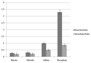
Fig. 1 The relative reaction rates  $[h^{-1}]$  and branching ratios for four different nanoparticles made by the same process (formation of ferrihydrite using an iron containing salt and reduction in hydrogen). Altering the initial salt had a significant impact of the overall reaction rate of CCI<sub>4</sub> with the particles in a water solution and significantly alters the branching ratio (the production of CCI<sub>3</sub>H). Data extracted from [24].
